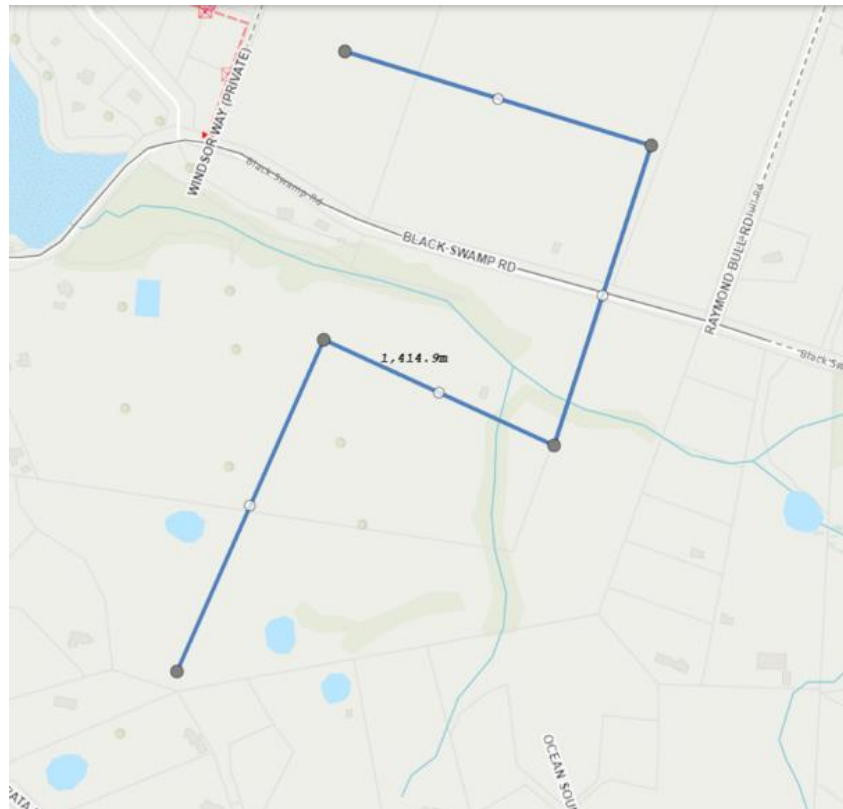
Figure 6: Potential fire reticulation layout
