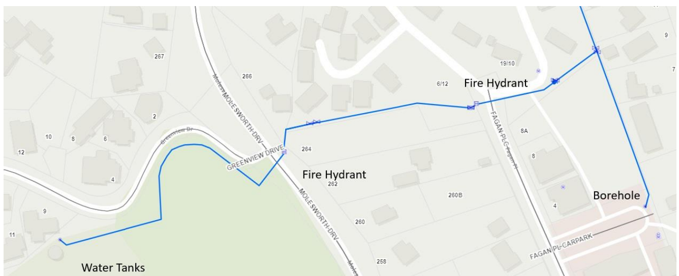
Figure 4: Water reticulation (Borehole to timbertanks, with two fire hydrants).
